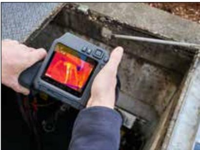
180° rotating optical block and bright 4" LCD make the T500-Series easy to use in any environment
