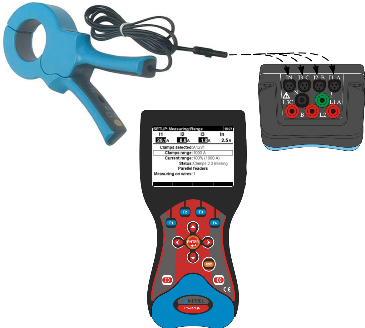
Figure 2: Current clamps A 1281 - connection to the measuring instrument
