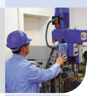
The MI 3121H Smartec 2,5 kV Insulation / Continuity is the portable measuring instrument for complete diagnostic testing of insulation and continuity measurements. Due to insulation resistance measurement with the test voltages up to 2.5 kV (measuring range is up to 100 G $\Omega$ ) and calculation of PI and DAR indexes the instrument is ideally suited for testing insulation of cable lines, current and voltage transformers, electric motors, etc.
