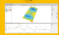
The clear graphic representation of the measurement results and extensive integrated evaluation and post-processing options support you in interpreting the measurement data. 3D animation, identification of resonances via cursor, Bode plots, deflection shape display in volume or sections are among the standard tools for vibration analysis.
